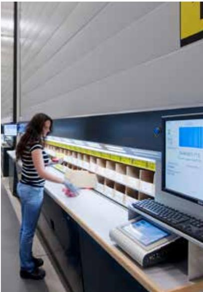
The Industrial Paternoster (IPN) Vertical Carousel saves time and money by optimising picking processes and minimising picking errors. It requires up to 75% less floor space compared to conventional warehousing solutions.
