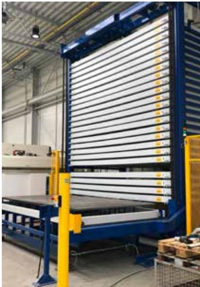
GMH Tower Storage Machines are designed for storing and handling of various types of heavy goods, especially material made of metal.
